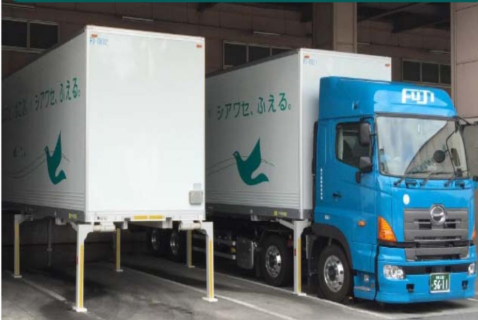
Nitori was awarded for the innovative introduction of the “Swap body container”, which allowed the loading platforms to be desorbed from the truck head. This system realize efficient high rotation which lead to the cost reduction of transportation and provided positive impact in labor environment
